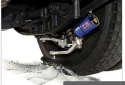
**Compact Solution-** Developed for vehicles with limited mounting space— (pneumatic suspension, low tires) air up, air down system; no spring **3 UNIQUE SYSTEMS**
